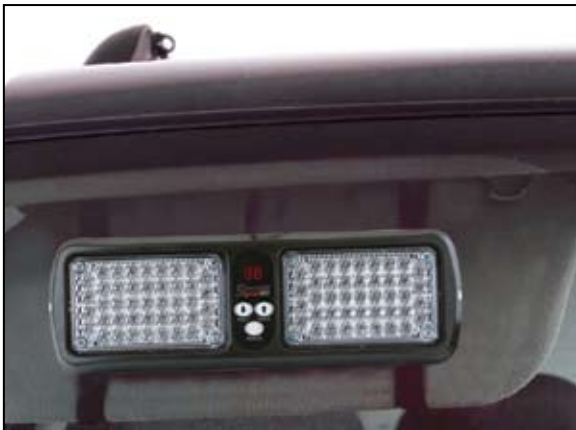
Perfect for undercover vehicles, light cannot be seen with the visor in the up position.
